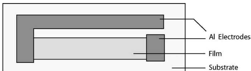
Figure 1 Evaporated planar device on substrate for thermoelectric power measurements.
